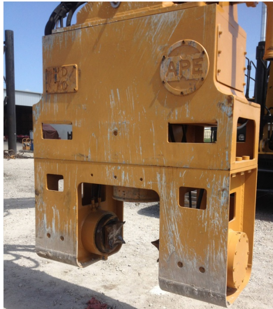
Photo 5 - APE Rotary Drive Head for Helical Piles
