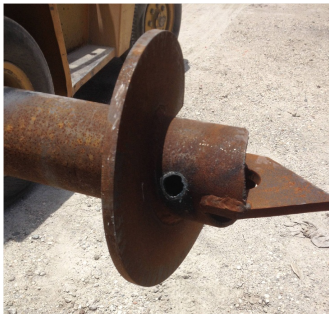
Photo 3 – Helical Pile Tip with Grout Holes
