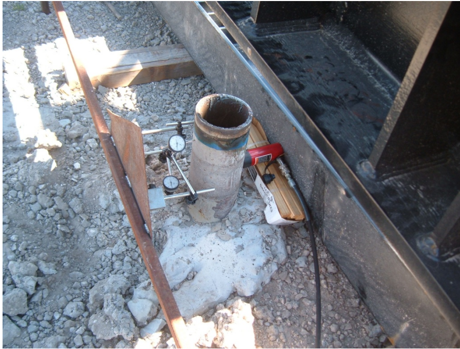
Photo 8 – Load Frame Setup for the Lateral Load Test
