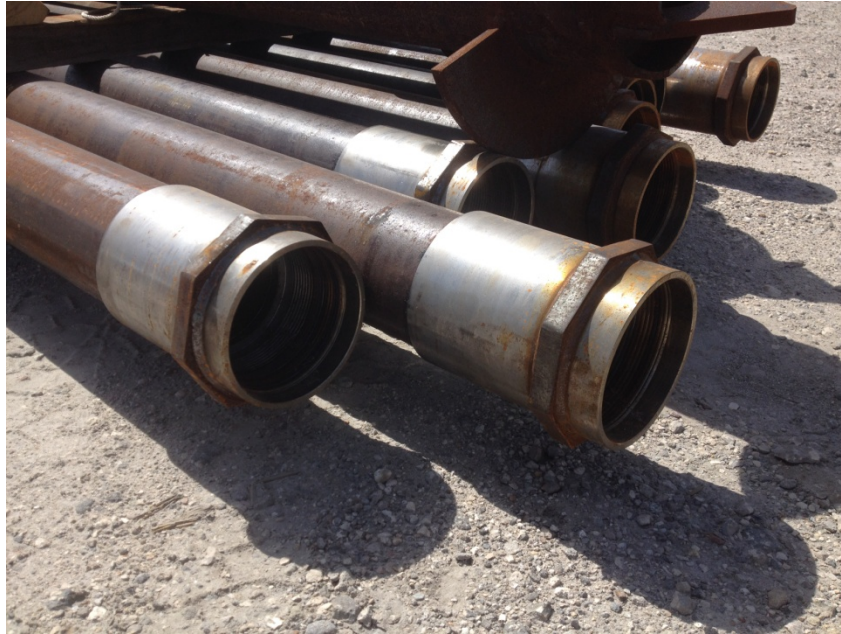
Photo 2 - Threaded Coupling at the Top of the Pipe Section
